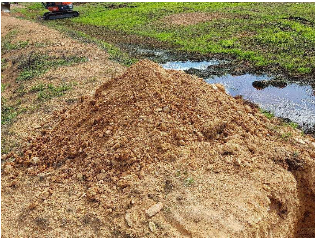
Image 7.3.1.2 View of natural soils encountered at TP37
