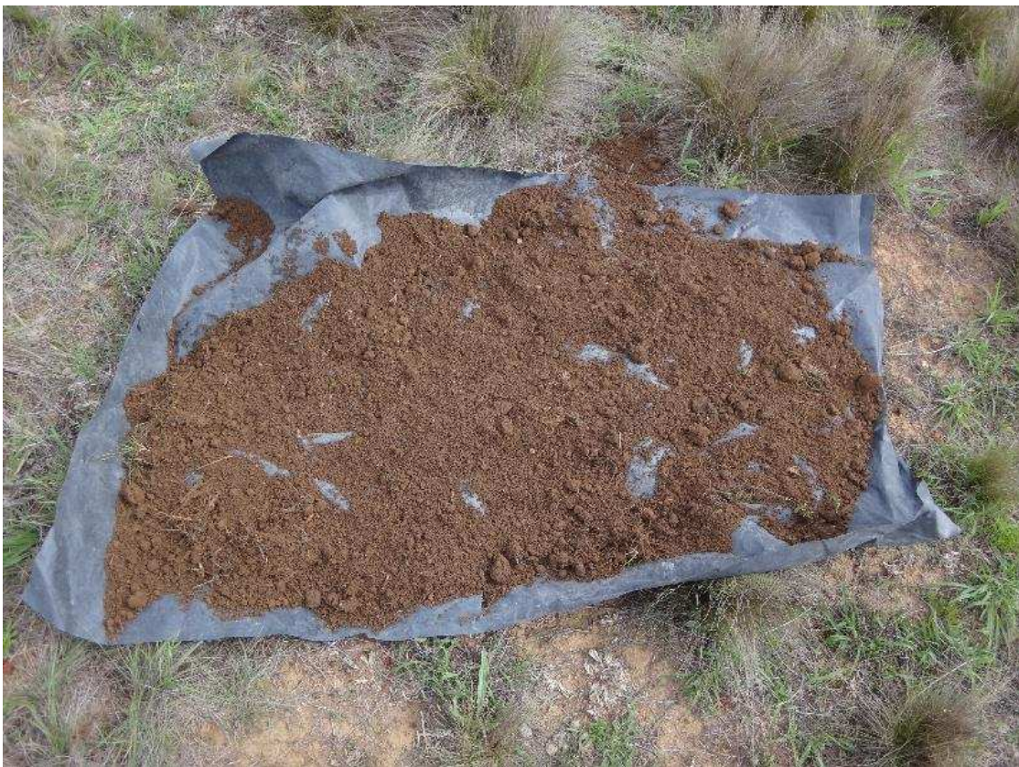
Image 7.1.4 View of asbestos field screening in progress at SS20
