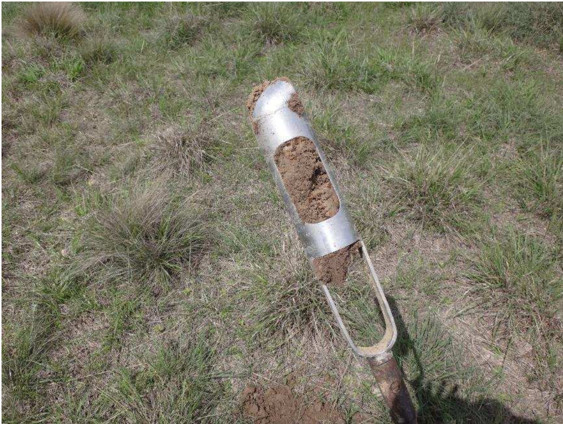
Image 7.1.5 Soil in the auger at ABC03
